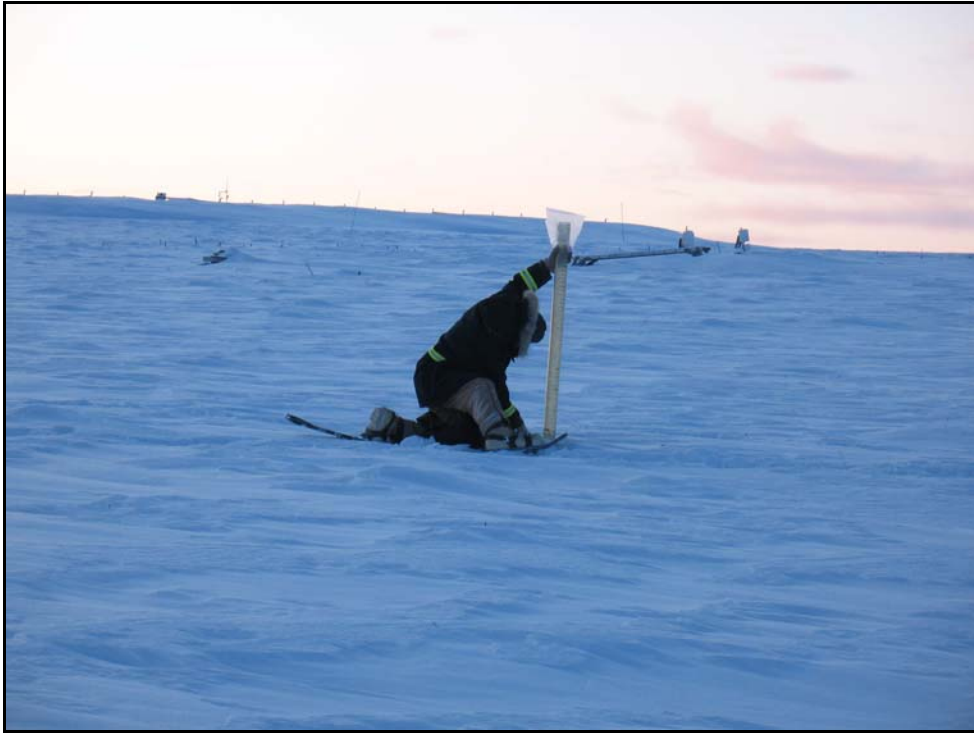
Figure 4. Jeff Derry getting ready to invert an Adirondack snow sampler to empty snow sample into plastic zip-lock bag. Site located due south of Toolik Research Camp. Photo by M. Lilly, November 21, 2009.
