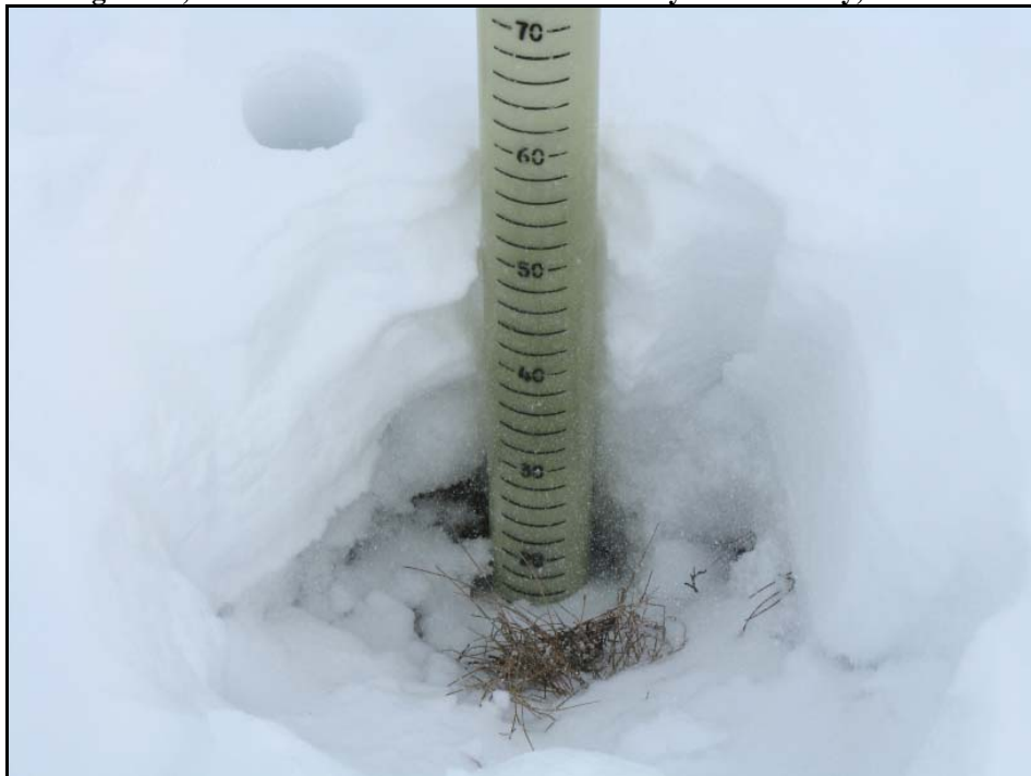
Figure 3. Adirondak snow tube inserted to snow/ground interface and snow depth recorded.
